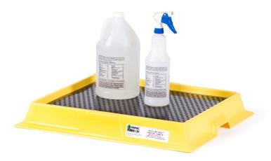
The precise work that occurs in a lab requires tailored containment found in the ENPAC Poly-Labtray. Its plastic construction is very chemically resistant, while the design catches overflows of liquid and powder chemicals during standard lab operations. The large surface can hold up to four 1-gallon bottles, while the sump holds a generous 2.5 gallons.
